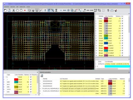
DWG measurement window with filters by layers and entity types
